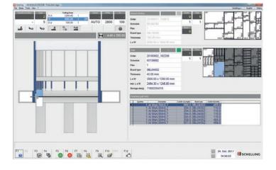
MCS Evolution also displays the current cutting plan, cut in process, the order and the material on the screen. The newly developed optical power display aids easy sight monitoring of the saw motor power.
