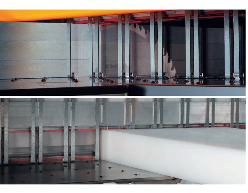
The design of chip guiding and extraction systems are some of the most important requirements for clean and precise cutting. IMA Schelling has integrated designs into the fk 6 / fk 8 that ensure almost one hundred percent removal of the chips generated by the cutting process.
