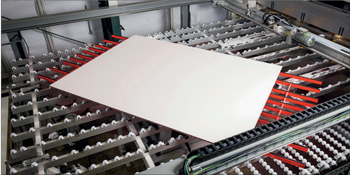
The turning device has been developed for automatic loading cut-to-size machines and angular systems
