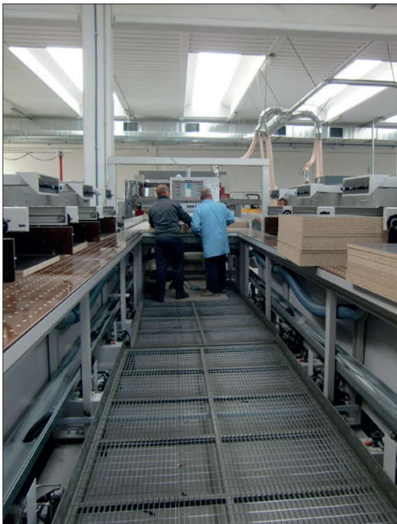
The turning device has been developed for automatic loading cut-to-size machines and angular systems
