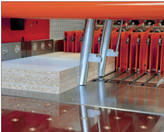
Even high books can be easily aligned to ensure the highest angular accuracy
