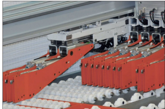
Two individually operating feeders that position the material independently of each other in the saw
