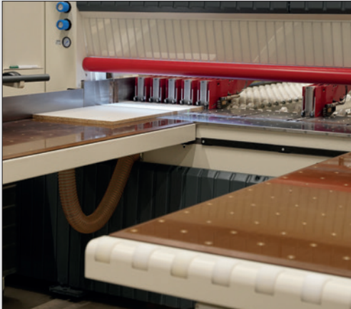
The air floatation table is always where it is needed at the moment
