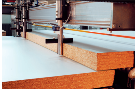
Automatic loading at the lifting table
