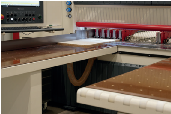
The air floatation table is always where it is needed at the moment
