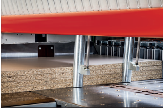
Double strip aligners ensure highest angular accuracy, even with thin panel strips
