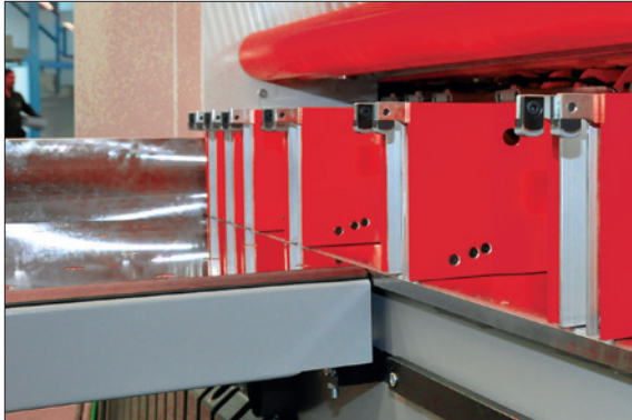
With the help of the clamps, the panels are transported directly to the saw and the air floatation table
