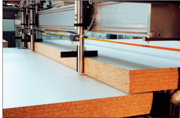
Automatic loading at the lifting table
