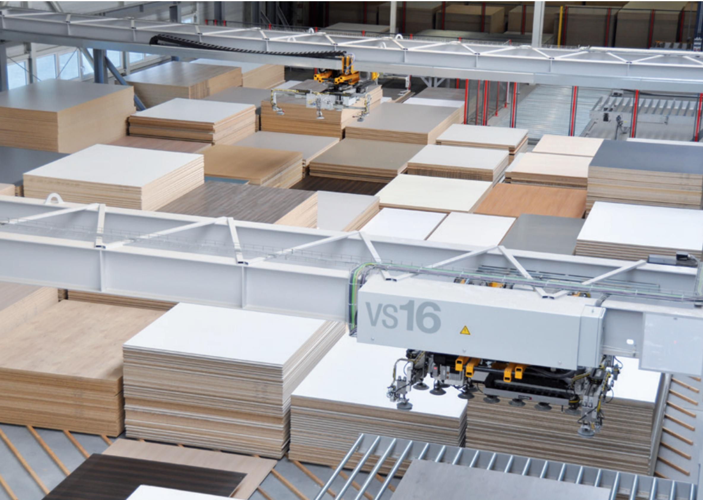
A practical development which ensures a further leap in productivity for cutting panels to size: the Schelling area storage system makes an important contribution toward increasing production capacities up to 100 %, while saving valuable time and expensive storage space at the same time.
